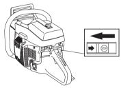
Stop the engine by switching off the ignition. (Move the ignition switch to stop position.)
